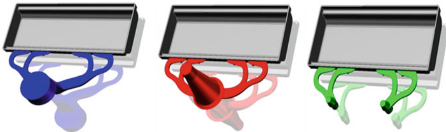
Fig. 12.16 Difference in processes allows different gating systems
